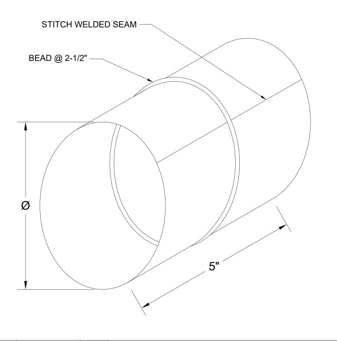
SPIRAL PRODUCED TO SMACNA STANDARDS. CONSULT SMACNA DUCT CONSTRUCTION MANUAL FOR CORRECT GAUGE FOR YOUR APPLICATION.
