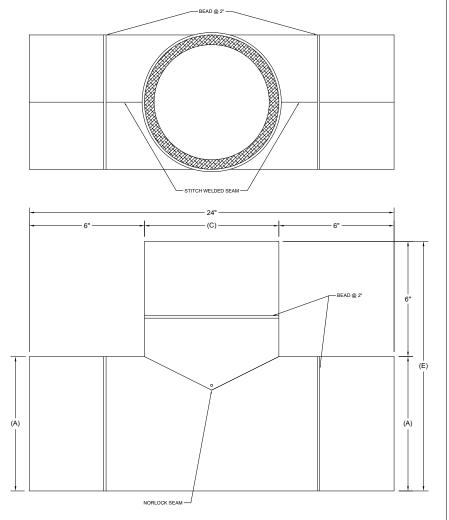
SPIRAL PRODUCED TO SMACNA STANDARDS. CONSULT SMACNA DUCT CONSTRUCTION MANUAL FOR CORRECT GAUGE FOR YOUR APPLICATION.
